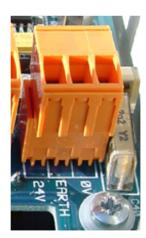
Remove the detector cover by unfastening the four screws at the front of the unit and detach the power supply terminal block. This is on the small fan relay board located at the top left with the detector held with the serial port at the bottom of the unit.
