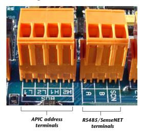
To connect the signal wire, lead a suitable wire type (RS485 cable 9841, 120 ohm screened twisted pair or equivalent) through the second cable gland and tighten it into position with about 35mm of cable from the bottom of the cable gland.
