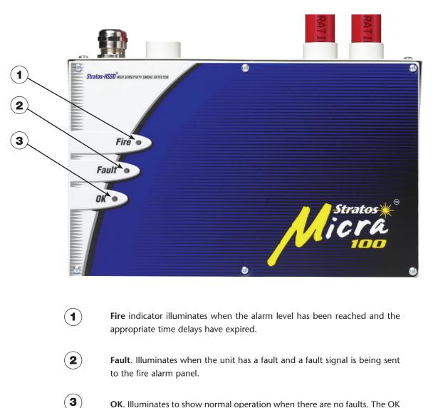
**OK**. Illuminates to show normal operation when there are no faults. The OK lamp will flash during the 15 minute Fastlearn<sup>™</sup> period when the detector is first learning about its environment.
