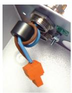
Each detector is supplied with a pair of RF suppression ferrite rings. To ensure compliance with all relevant EMC requirements, the conductors of each cable should be wound once around a ferrite as shown here before entering the relevant connector. Power conductors should be on a separate ferrite, but different forms of signal conductor (e.g. RS485 and relays) can share the same ferrite.
