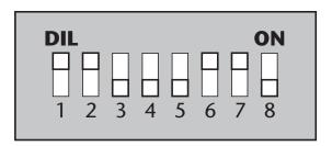
The address equates to 01100011 in binary, or  $(1 \times 1) + (1 \times 2) + (0 \times 4) + (0 \times 8) + (0 \times 16) + (1 \times 32) + (1 \times 64) + (0 \times 128) = 99$ .
